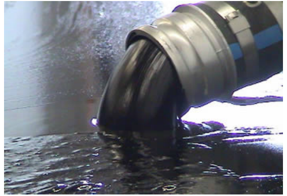
Condensate is used to thin heavy oil so that it can easily pass through pipelines.
